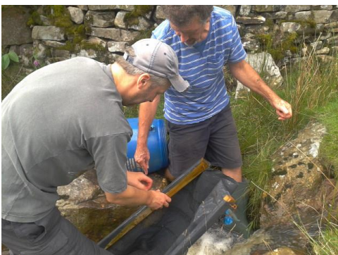
Flow gauging at Nant yr Hafod, one of the Phase 2 streams. Water from the stream is captured in the tapered plastic sheet with the aid of strategically placed sandbags, then directed into the blue 30L barrel.
