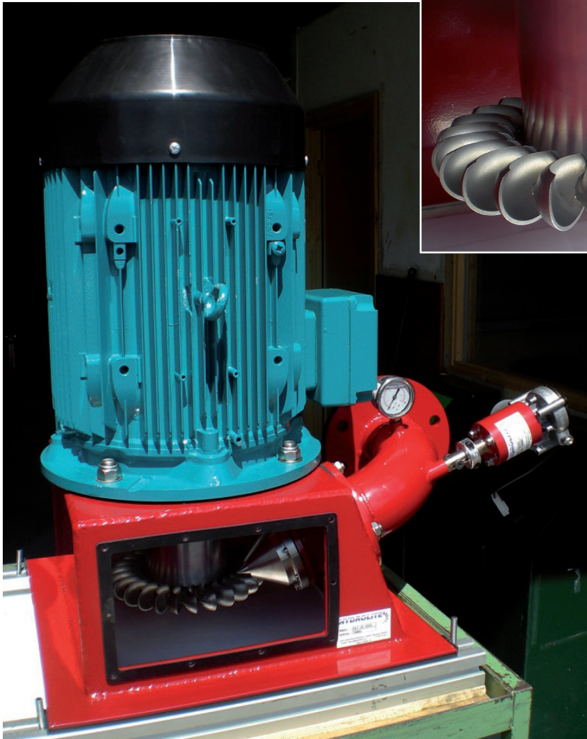
A typical Turgo turbine, left, with a close-up of the spear valve and runner, above
